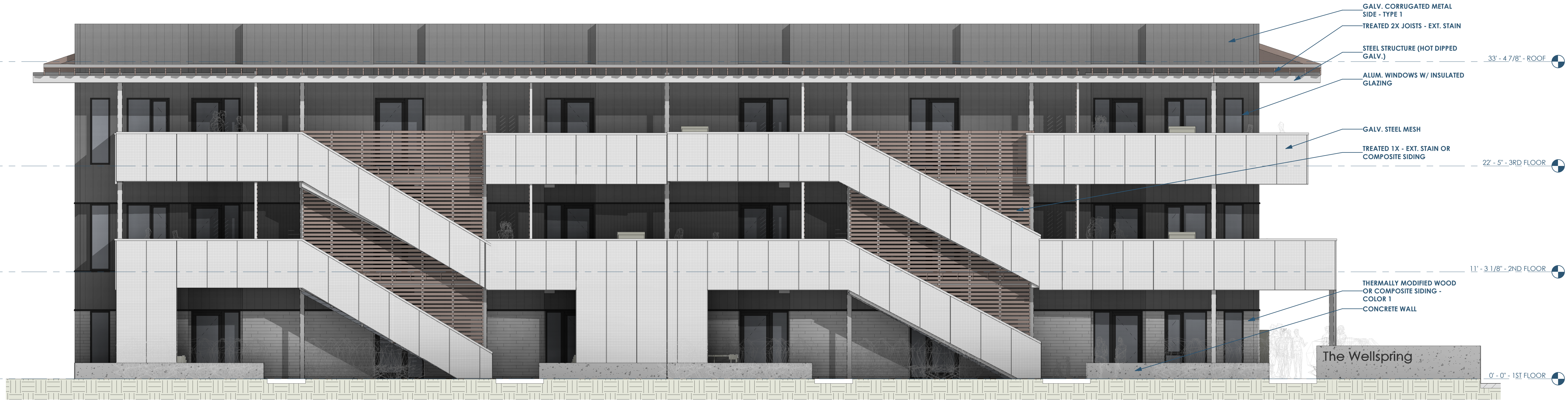
1 BUILDING ELEVATION - NORTH Q1-A201 3/16" = 1'-0"
