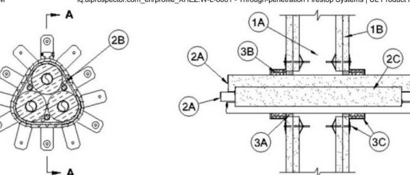
1. Wall Assembly — The 1 or 2 hr fire-rated gypsum board/stud wall assembly shall be constructed of the materials and in the manner specified in the individual U300 or U400 Series Wall or Partition Design in the UL Fire Resistance Directory and shall include the following construction features:
