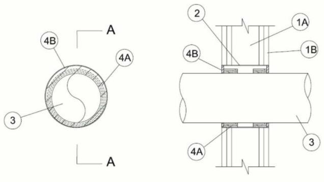
SECTION A-A The hourly F and T Ratings of the firestop system are equal to the hourly fire rating of the wall assembly in which it is
