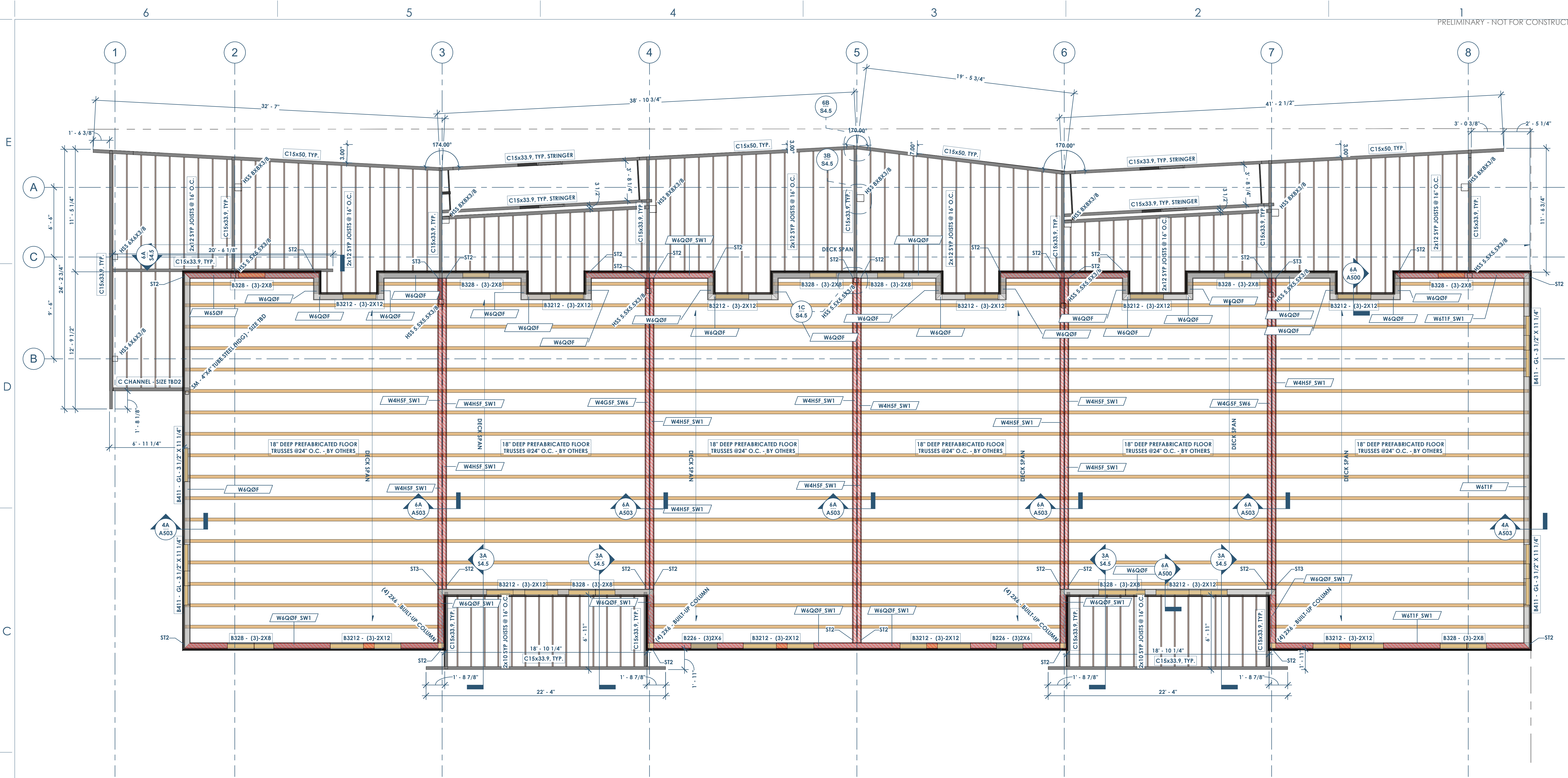
68 S0.2 FRAMING PLAN - 2ND FLOOR 1/4" = 1'-0"
