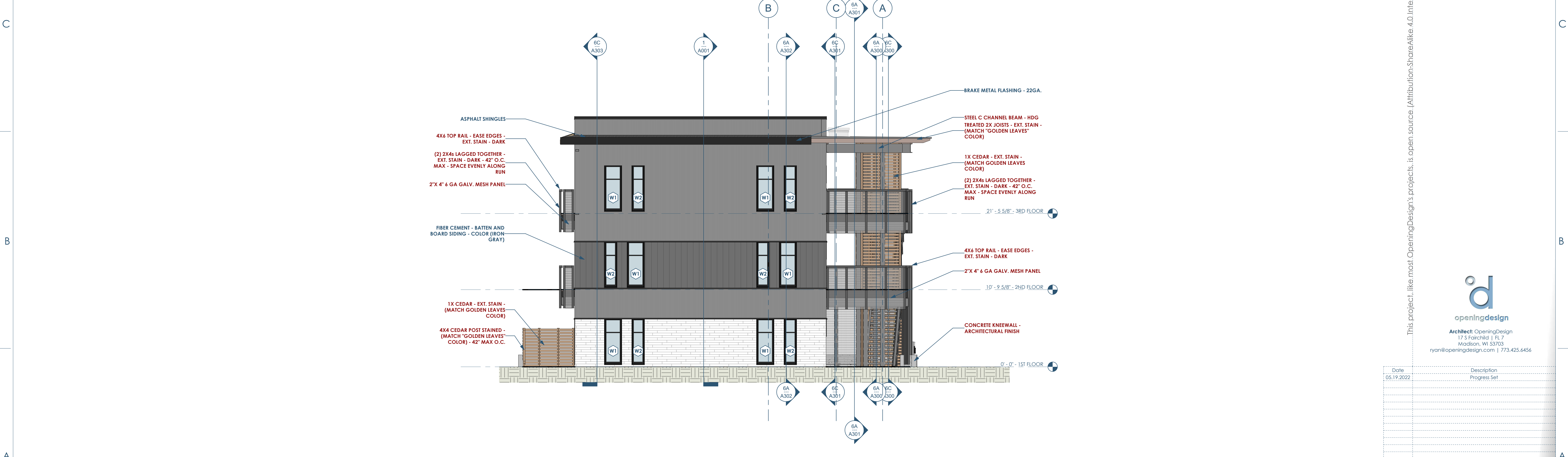
6A A201 BUILDING ELEVATION - EAST 3/16" = 1'-0"
