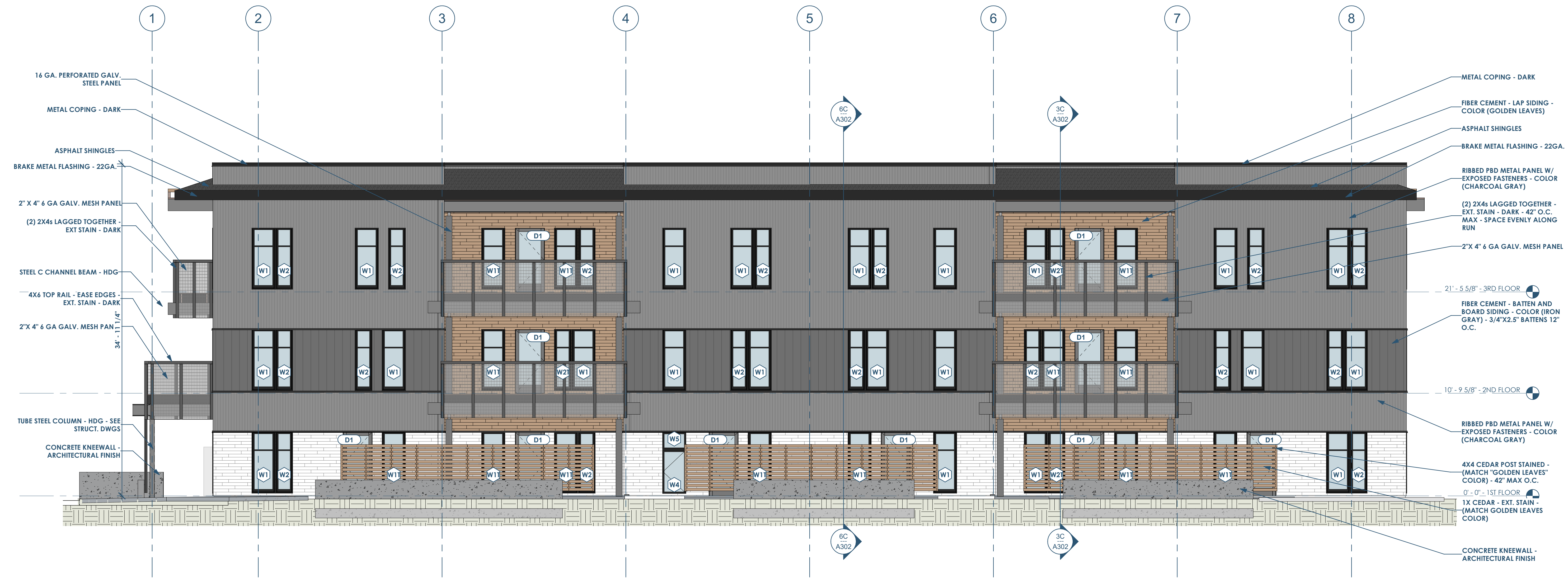
6C A201 BUILDING ELEVATION - SOUTH 3/16" = 1'-0"
