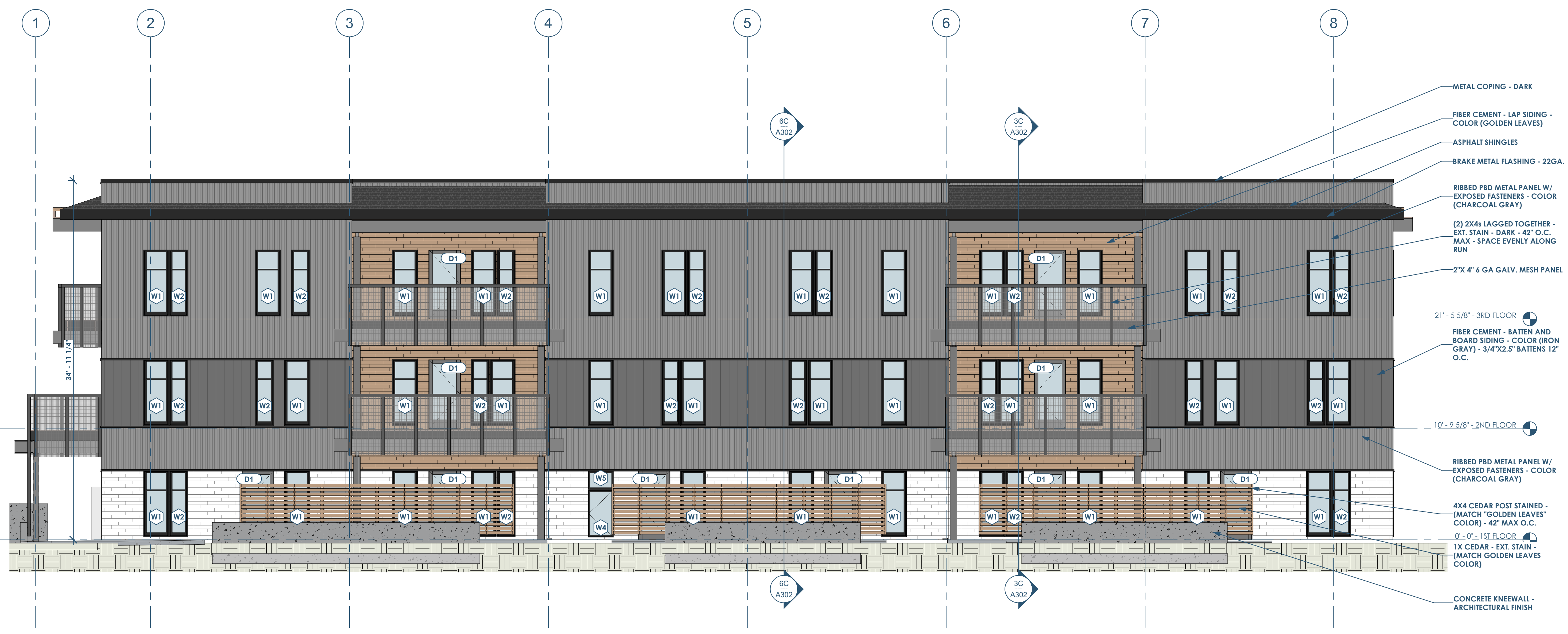
6C A201 BUILDING ELEVATION - SOUTH 3/16" = 1'-0"
