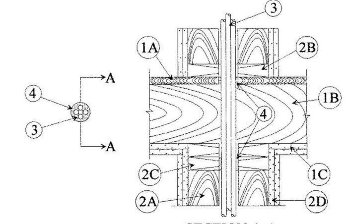
1. Floor-Ceiling Assembly — The 1 or 2 hr fire-rated solid or trussed lumber joist floor-ceiling assembly shall be constructed of the materials and in the manner specified in the individual L500 Series Floor-Ceiling Designs in the UL Fire Resistance Directory. The general construction features of the floor-ceiling assembly are summarized below:
